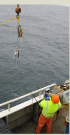
Figure 10: Launching of underwater video camera
